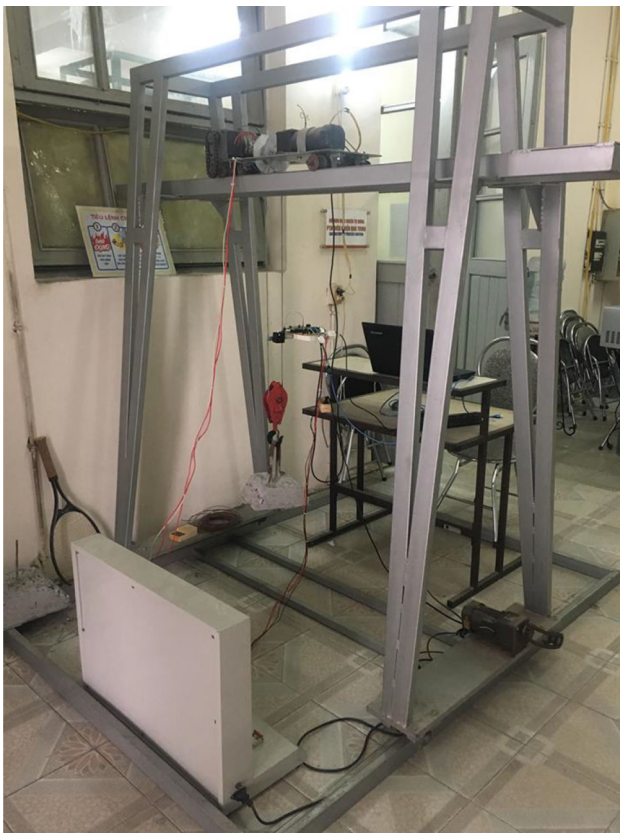
Fig. 2 The 2D overhead crane control system in laboratory
